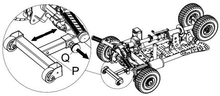
WARNING ! To prevent the scooter from tipping backwards the anti-tip frame must be locked in the maximum extended position.
