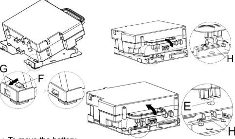
• To move the battery just pull up and move away.
