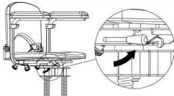
To turn the seat, lift and hold the turn release handle below the seat (as shown). This will allow the seat to turn.
