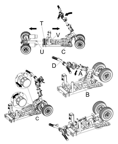
• Use one hand to hold the handle, and use the other hand to pull the lock pin knob (C) and turn it anticlockwise. Then fold the handle down until you hear the "click" of the locking pin fitting into position on the main frame.
