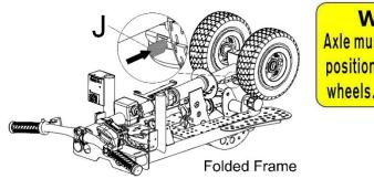
WARNING ! Axle must be securely locked in position after assembling front wheels. (Refer to user manual)
